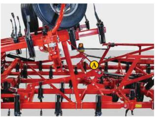
Figure 3.12 Wing Rest (5–Section) I
