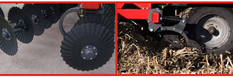
Two rows of double-mounted discs can be set for desired depth independent of the shanks. Concave razor blades are 24 inches (61 cm) in diameter and spaced 15 inches (38 cm) apart. The second rank of blades is offset from the first for effective spacing of  $7\frac{1}{2}$ -inches (19 cm).
