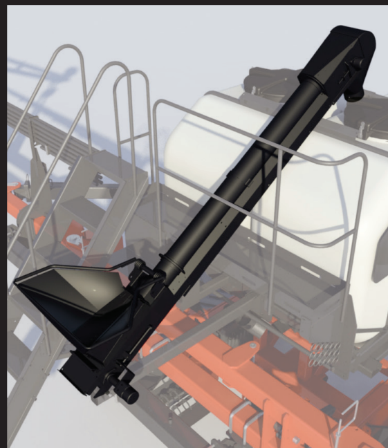
An optional 9' (2.7 m) cleated belt conveyor makes loading easy.
