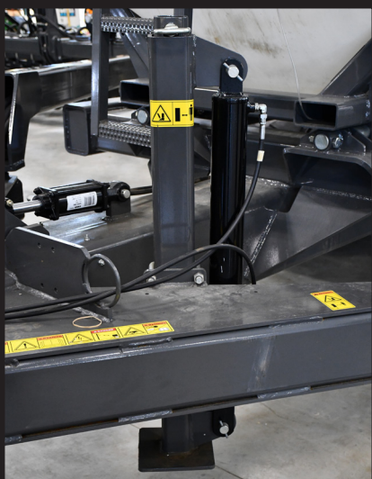
Hitch-mounted hydraulic jack makes hooking up easier.
