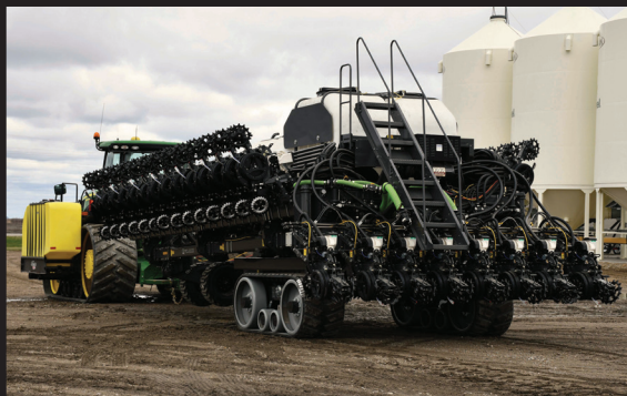
Tilt and rotate cylinders fold the toolbar for easier transport.
