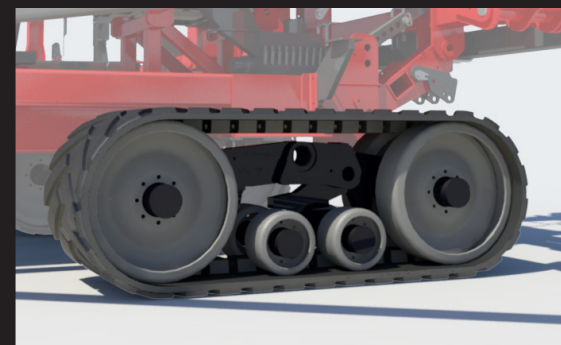
25" and 30" (64 and 76 cm) wide tracks reduce compaction and allow earlier entry into challenging field conditions.
