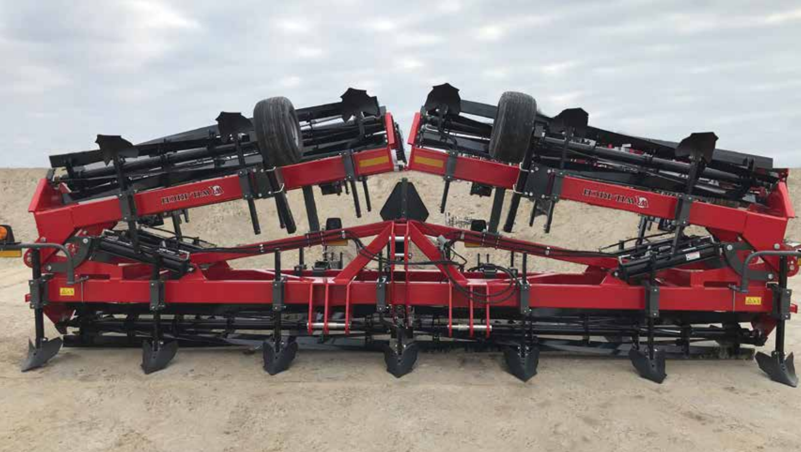
Above: The Wil-Rich 12-Row 1500 Series Bedder Finisher has four wing fold cylinders and folds to 20'5" ft for easy transport.
