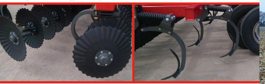
Two rows of double-mounted discs can be set for desired depth independent of the shanks. Concave razor blades are 24 inches (61 cm) in diameter and spaced 15 inches (38 cm) apart. The second rank of blades is offset from the first for effective spacing of 7½-inches (19 cm).
