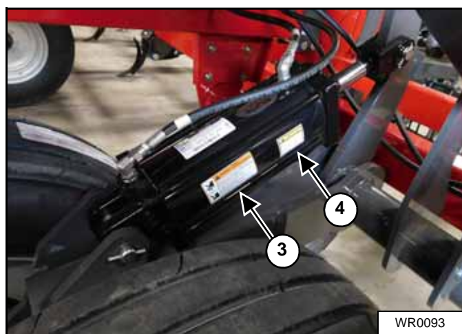
Left and right wheel lift cylinders.
