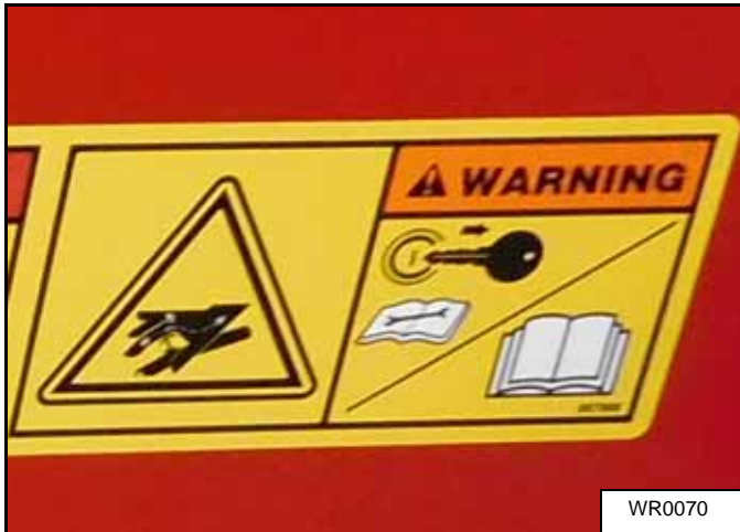
10. WARNING - Hydraulic hazard - P/N 997858
