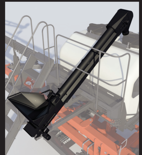
An optional 9' cleated belt conveyor makes loading easy.
