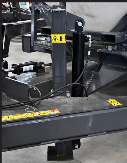
Hitch-mounted hydraulic jack makes hooking up easier.
