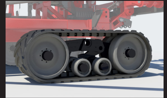
25" and 30" wide tracks reduce compaction and allow earlier entry into challenging field conditions.
