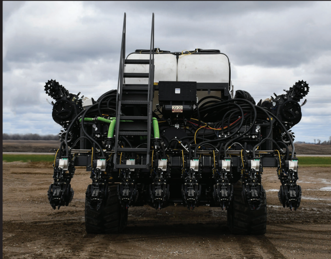
The 10K Planter Bar has rotating wings that fold forward for easy transport.
