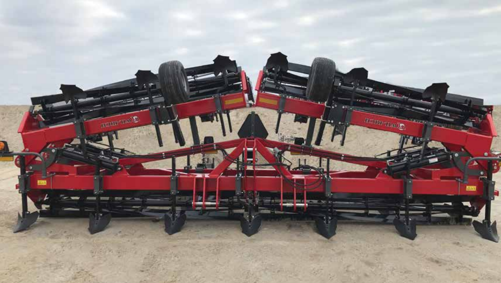
Above: The Wil-Rich 1500 Series Bedder Finisher has four wing fold cylinders and folds to 20'5" ft for easy transport.
