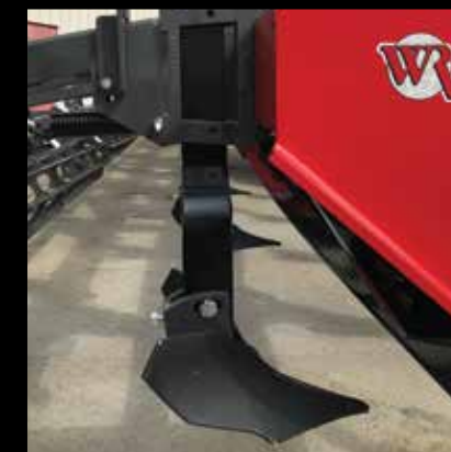
Bed shanks and optional furrowers penetrate the ground to break up soil and build a raised seedbed.
