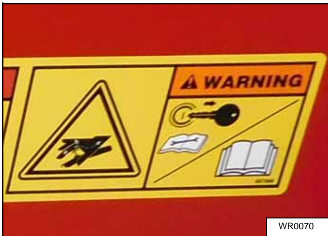
11. WARNING - Hydraulic hazard - P/N 997858
