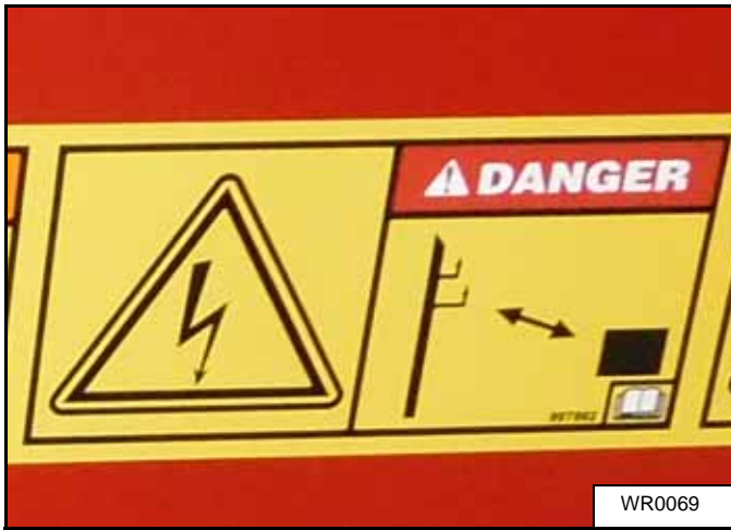
10. DANGER - Electrocutation hazard - P/N 997862
